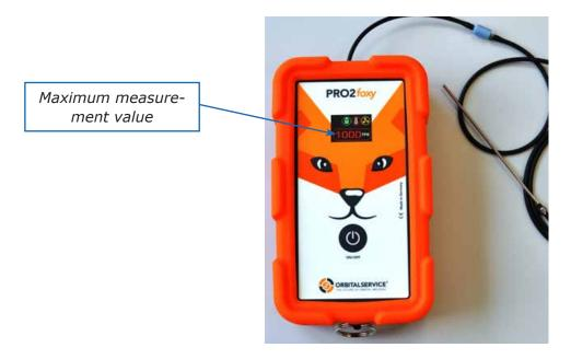
When a value below the pre-programmed 30 ppm is measured, an acoustic signal is transmitted from the device. This value can be reprogrammed with an Android smartphone.
