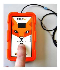
When turned on, the device will transmit an acoustic signal and show a home screen (seen below) for 3 seconds. This screen displays serial number, software version and signal ppm. The shown ppm value determines the threshold where the device will display the value with green color and transmit an acoustic signal. The pre-programmed value is 30 ppm.
